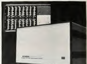
SAMPLING CONVERTER —Studer's SFC 16 digital sampling frequency converter for professional use makes it possible to transfer digital audio programs between recorders and other systems with conflicting sampling frequencies. The unit does not require programming. It operates strictly under control of the clock signals.
